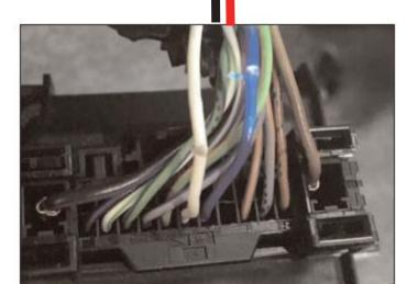
Note: Vehicles Equip. with gateway connector on back of OBD2 solder cruise Red CAN high wire to Blue wire in position 20. Solder Black CAN low wire to White position 19.
