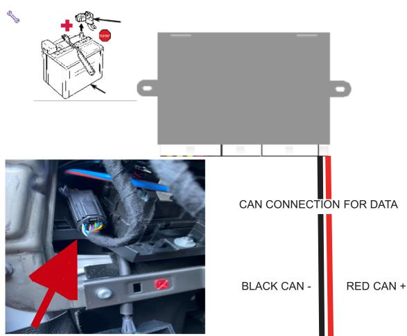
Note: Vehicles Equip. with 12 Inch Radio Screen will need to locate 21 pin plug behind electric parking brake switch under dash. Solder Red CAN wire to Blue wire in pin 2 and solder Black CAN wire to White in pin 1.
