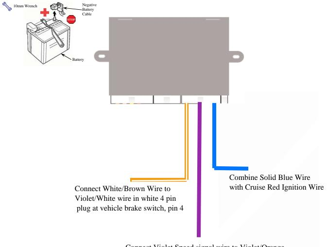
Connect Violet Speed signal wire to Violet/Orange wire in gray 6 pin plug at Customer Interface Connector located under drivers seat, pin 4. or Violet/Orange wire in gray 8 pin plug, pin 5 at same location.
