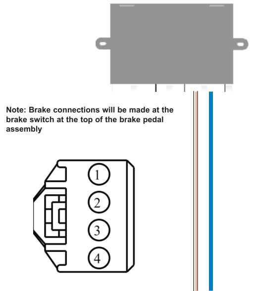
Connect the WHITE/BROWN Rostra negative brake wire to the VIOLET/WHITE at the brake switch of vehicle Position 4.
